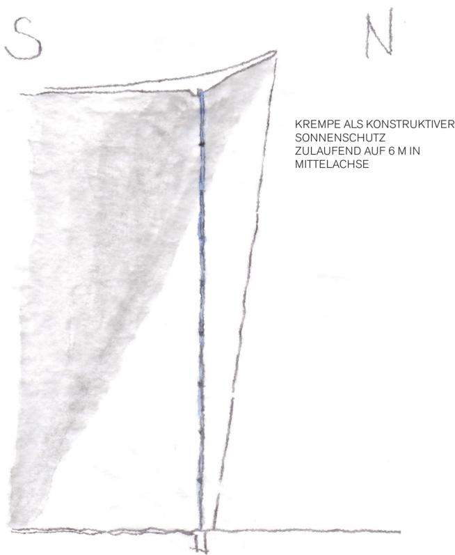
KREMPE ALS KONSTRUKTIVER SONNENSCHUTZ ZULAUFEND AUF 6 M IN MITTELACHSE
