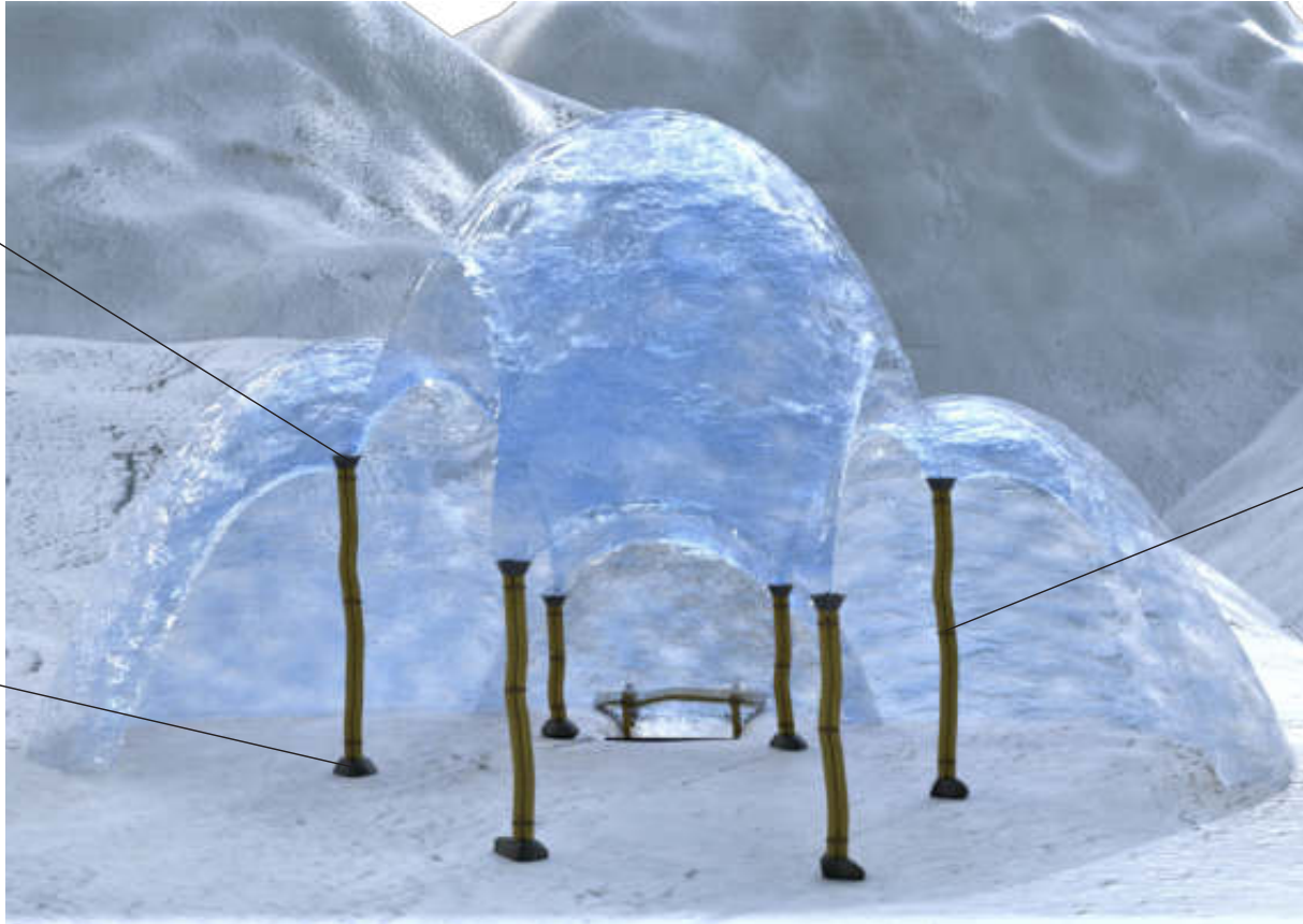
connection between Ice shells and bamboo columns via metal hopper plugged into the bamboo canes
