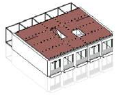
8. Massivholz Decken + X-Fix C + Stiege
