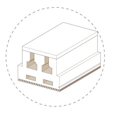
Cross Laminated Timber Floor Slab Detail
