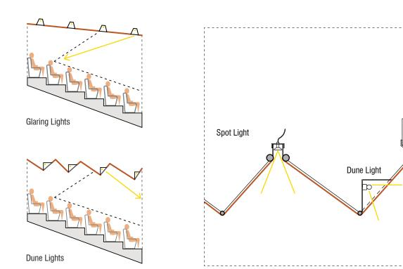
Concept Diagrams non glaring ceiling lighting / lights, ventilation and acoustic insulation conceiled behind ceiling
