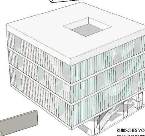
KUBISCHES VOLUMEN, STAHLBETONSKELETTKONSTRUKTION MIT UMLAUENDER GLASFASSADE ALS THERMISCHE HÜLLE
